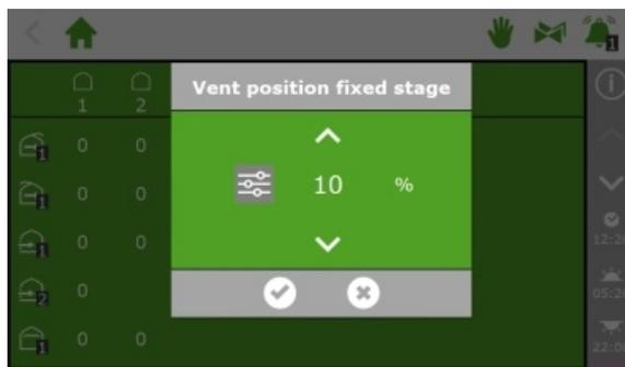
Figure 3-5: Configuring fixed position settings
