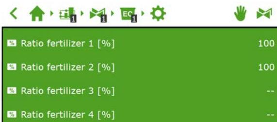
Figure 5-4: Dosing ratio of fertilizers
