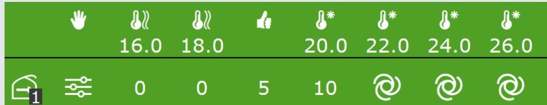
Figure 4-10: Automatic ventilation control on leeward side from 22°C.
