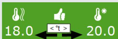
The desired ambient temperature is between 18.0 and 20.0°C. The first heating stage starts when the temperature drops below 18.0°C. The first cooling stage starts when the temperature rises above 20.0°C.
